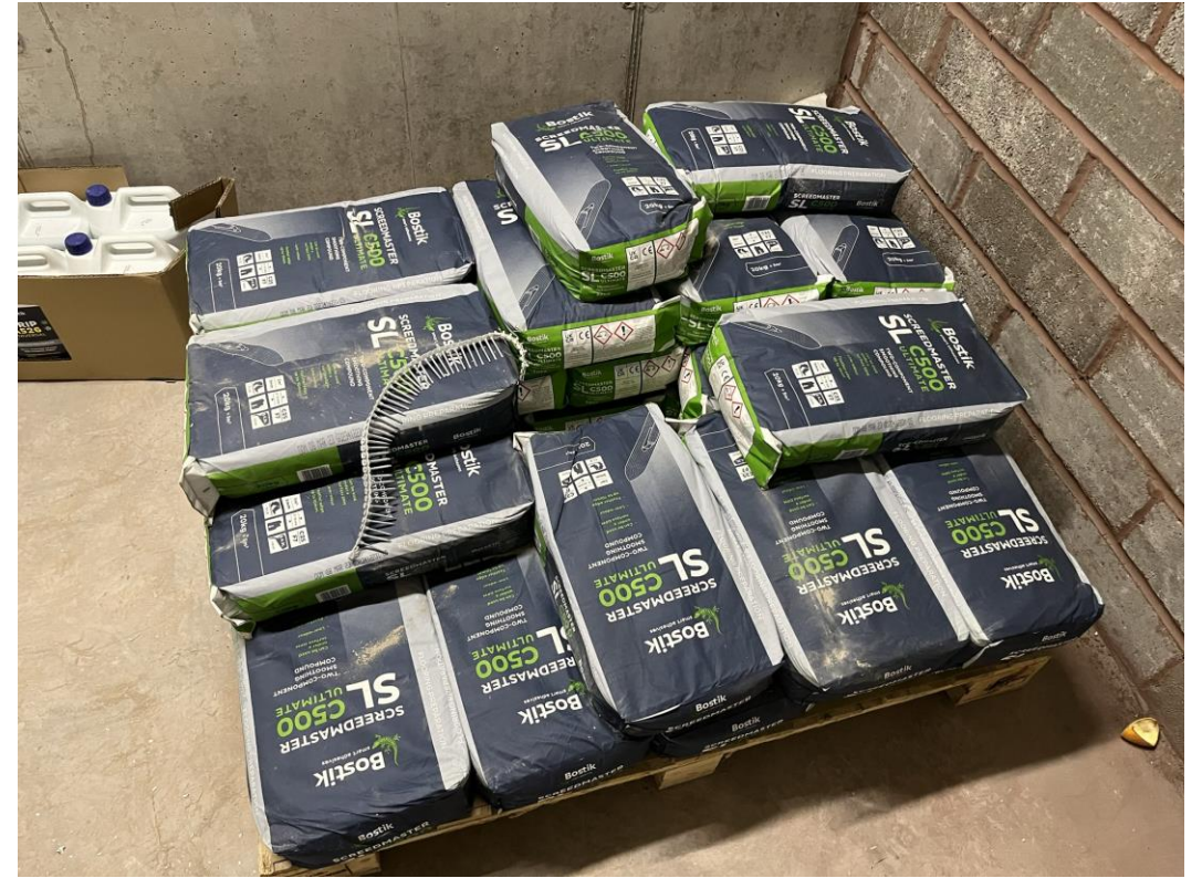
Materials: Self-levelling screed mix
