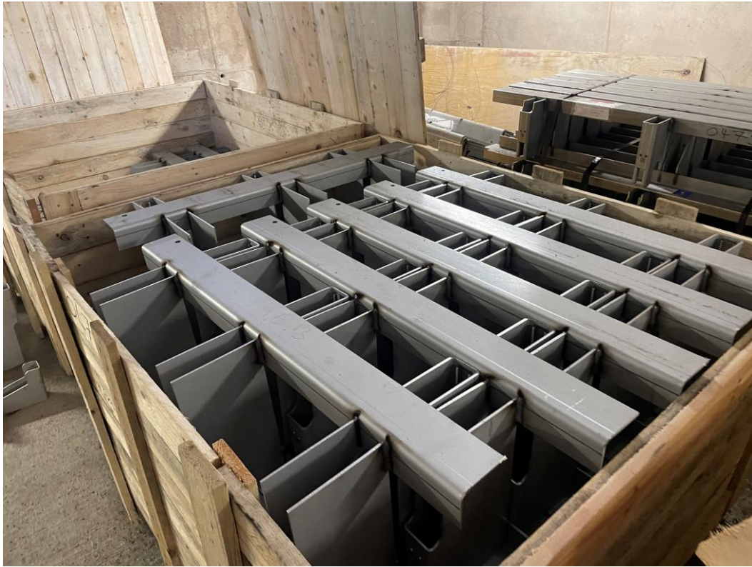
Brick angle supports
