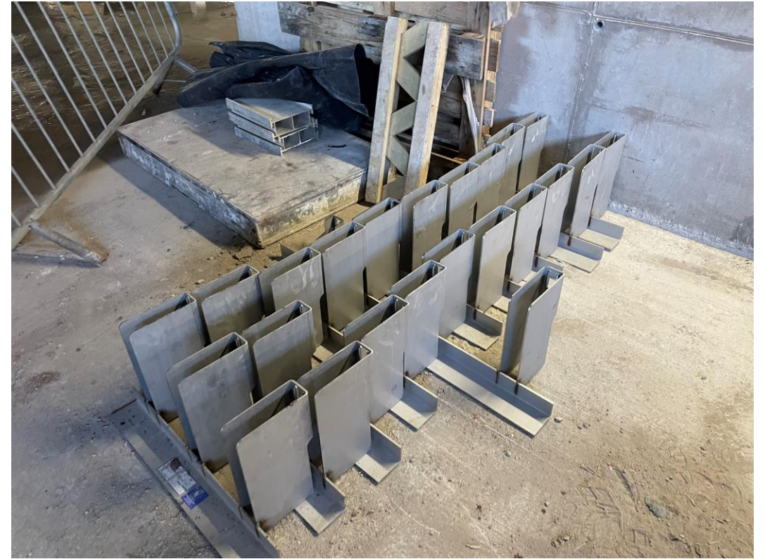
Brick angle supports
