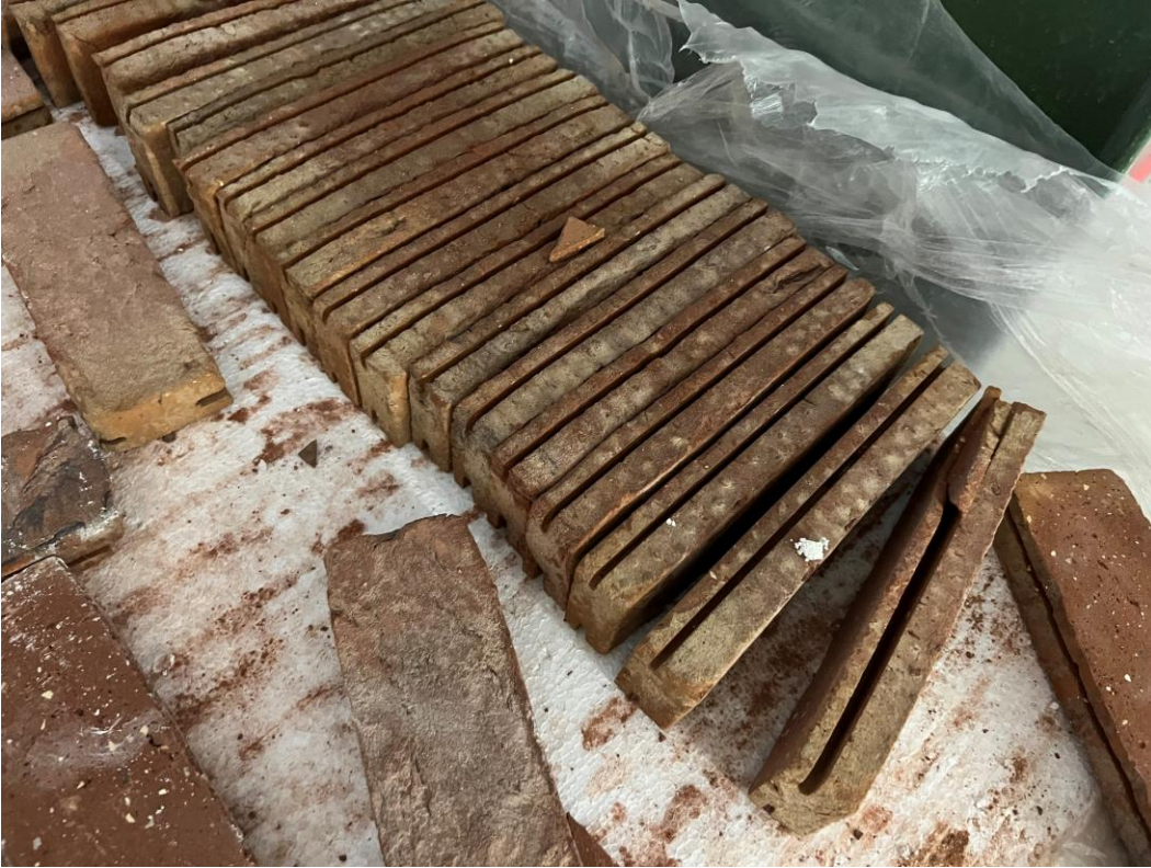
Materials Stored – Brick Slip
