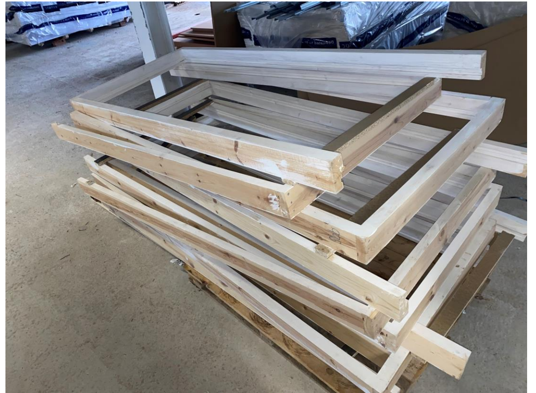
Material Storage – Door frames
